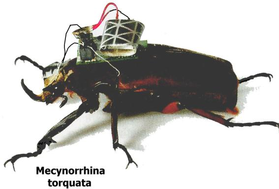
Figure 8.2.22 This beetle carries a miniature radio, controller, and battery and can be controlled in flight (Maharbiz and Sato, 2020)
